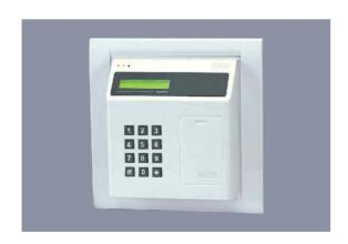
Solus Attendance Management System – SAMS<sup>™</sup> uses Time Prox or Time Smart terminals depending upon the tasks. All terminals are operated. Online with an Ethernet or RS 422 connection to guarantee the most current data transmission and data processing in SAMS<sup>™</sup> or in a superior ERP system. If the server is not available for data communication, the terminals automatically switch to Offline mode. The terminals save all entries and transmit them when the server is available again
